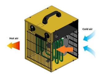
The device works on the principle offorced convection . The air flow is forced fan. Cold air is drawn in the back of the unit. Further washes flowing from the heater receives heat. The heated air is expelled in front of the heater. The device has a thermostat for the regulation temperatures 5-35  $^{\circ}$ C. The unit area equipped with thermal protection is acting automatically. The unit features: ventilation, heating with half the power, heating at full power. Device has cooling thermostat.
